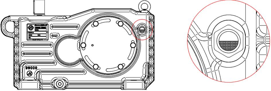
To check the oil level, verify that it is between the two notches (FIG. 5.4).
